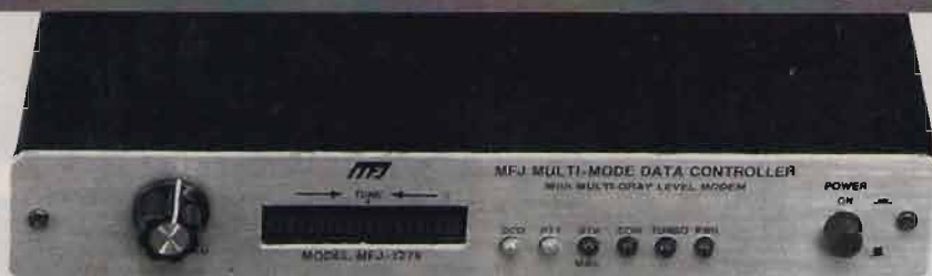
Multi-mode Data Controller - Computer Interface MFJ-1278
